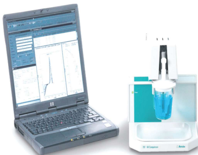
Fig 2: Trace metal analyzer Make - Metrohm, Switzerland. Model – 797VA
